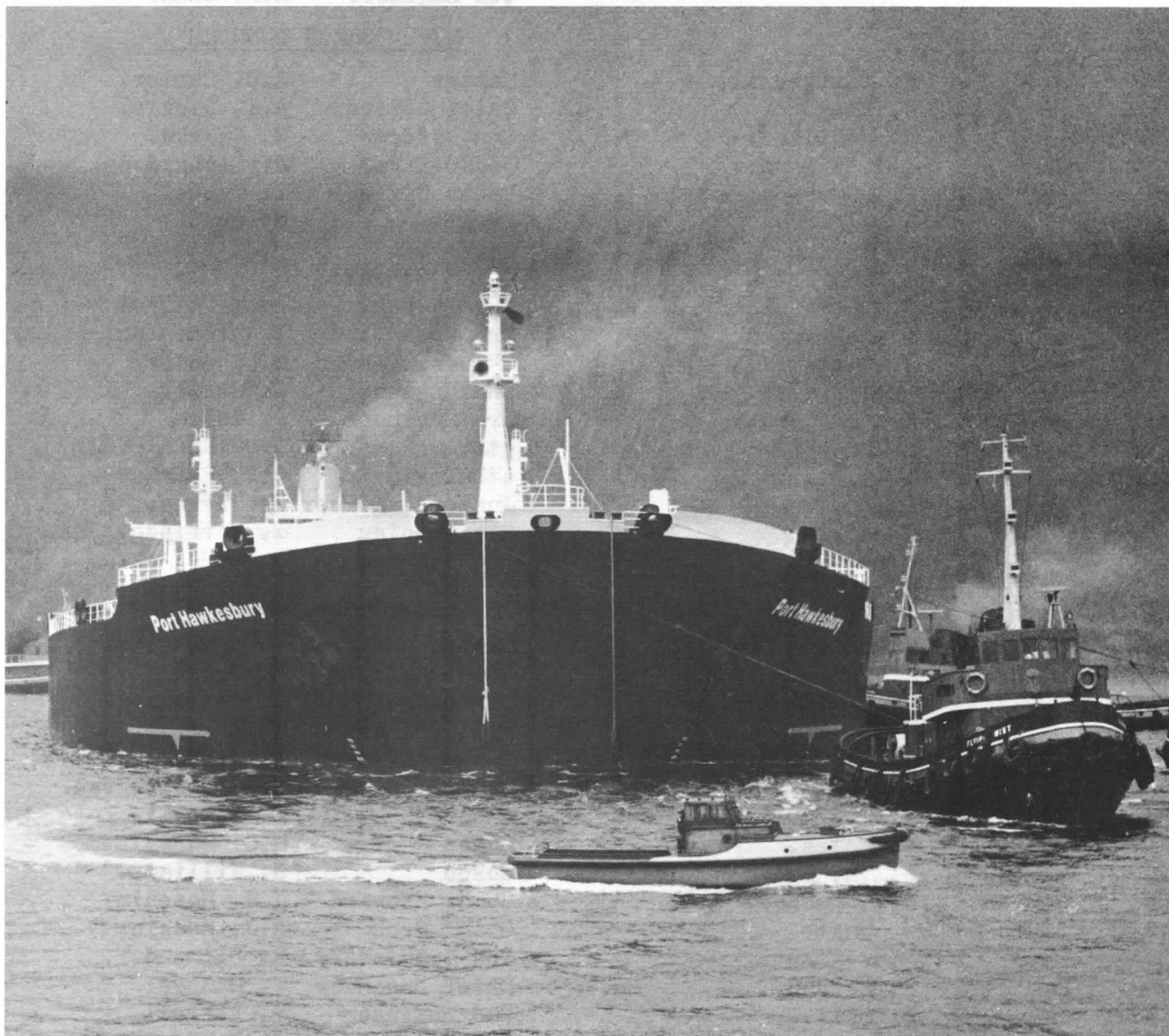
Bow-on view of the "Port Hawkesbury" approaching Finnart Oil Jetty, Loch Long. The bow draft markings show her drawing sixty-eight feet forward!
